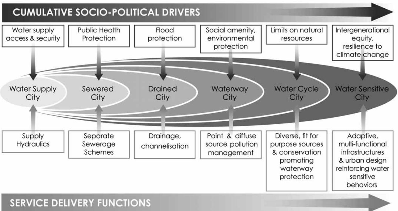
**Figure 1** – A transitions framework for urban water management that includes the concept of a 'water sensitive city' (from Brown *et al.*, 2008)
